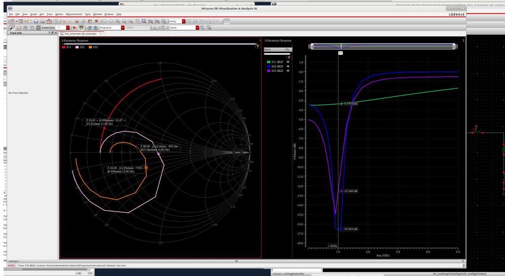
Figure 26: Part 5 – Images 3 & 4. Smith-chart trajectory (left) and |S_{11}| (right) for the series- C , shunt- L network.
