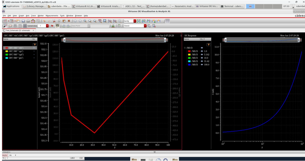
Figure 3: Part 1 – Image 2. Extracted V_{th} as a function of device width (finger count F ).
